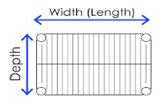
To ensure a shelf will fit onto an existing pole you need to measure the Shelf Collar which are the circles at the corner of the shelf.
